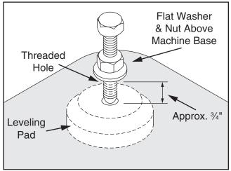
Figure 14. Leveling pad and bolt installed.
